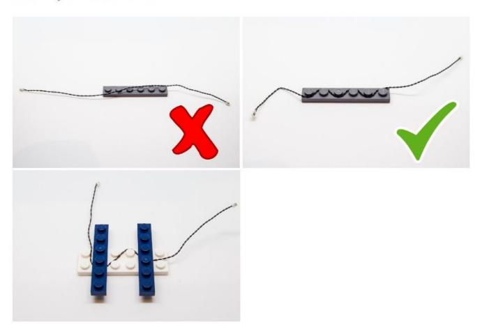
CAUTION: Forcing LEGO® to connect over a cable can result in damaging the cable and light.
